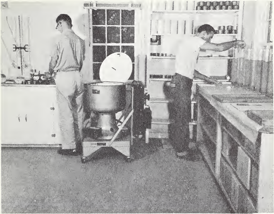
Figure 15.—In the laboratory a man on the left is weighing the soil sample while the man on the right determines texture (percent of sand, silt, and clay). The centrifuge that stands between them is used for studying soil moisture.
